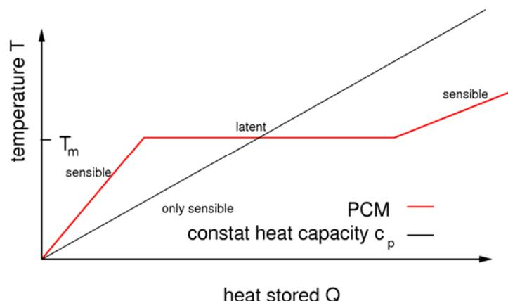
Figure 13 Difference between sensible and latent heat storage
