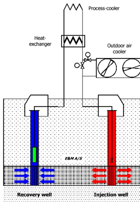
Figure 12 Principle of using an aquifer for a cold storage
