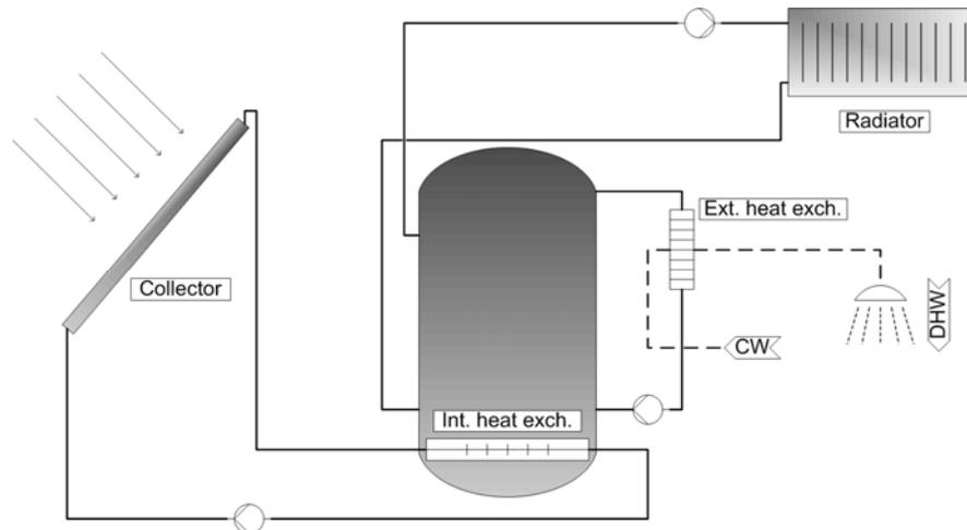
**Figure 11 Scheme of a state of the art solar water storage used for heating and domestic hot water**
