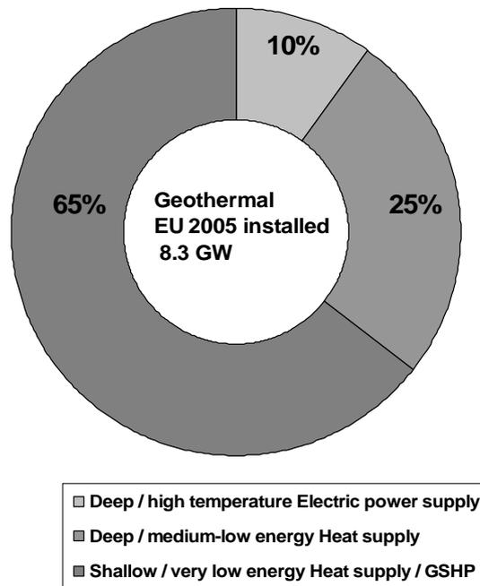
Figure 9 Installed geothermal energy capacity
