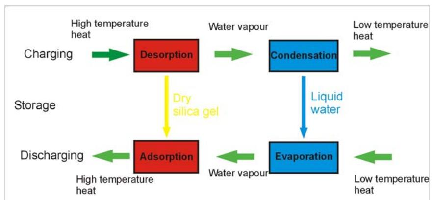
Figure 17 Working principle of an adsorption heat storage in a closed system
